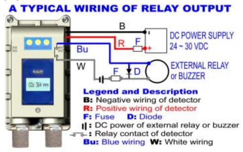
A recommend fuse is 0.2 A, the diode could be 1N4002 or 1N4004 in the above.
