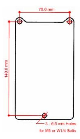
3. Due to the space is very small that is impossible to use wrench. Therefore, to use female expansion bolts on the wall or tap female screws on the steel plate and use external screw (male bolts) that can use the screw driver to install the gas detector and solve spacing problems. M6 sizes of bolts have a good tolerance than W1/4.
